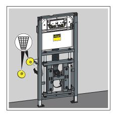
■ Remove the transport locks from the threaded rods and discard.
