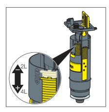
Set the small flush volume at the drain valve.
