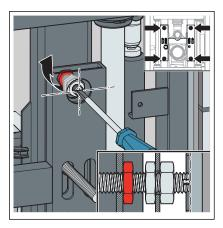
■ Tighten the rear threaded nut at all four points.
