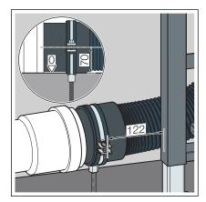
Alternative 1: Secure the drain elbow onto the wall or floor without the fixing material supplied, taking into account the fixing sizes.
