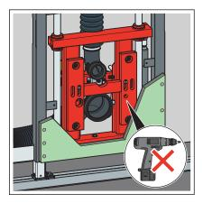
■ The plasterboard cladding panels must not be screwed together with the height-adjustable internal frame!
