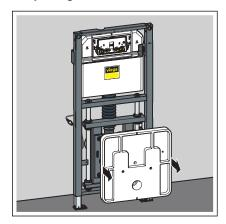
Remove the mounting template from the element.
