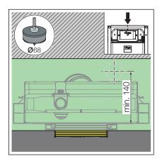
■ If the actuation button is mounted above the cistern, maintain a minimum distance of 140 mm to the centre of the concealed socket.
