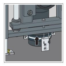
Alternative 2: Vertical pipeline through the bare concrete floor Screw the fixing elbow on the element.
