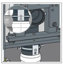
**INFO!** Installing pipelines vertically through the bare concrete floor is only possible with the drain elbow (model 8095, Art. No. 713744). The screed height must be at least 85 mm.
