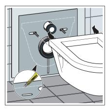
Install the WC ceramic and sound insulation panel.
