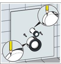
Mark the insertion depth of the flush pipe and drainpipe.
