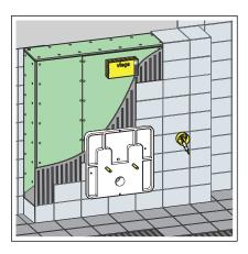
Tile up to the mounting template and concealed socket.
