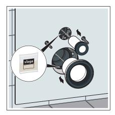
Coat the flush pipe and drainpipe with silicon grease and insert them.
