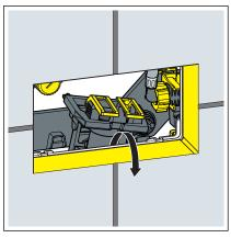
■ Remove the drain valve through the revision opening.
