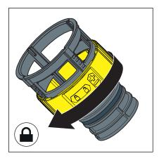
Lock the flushing throttle.
