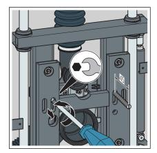
■ Unscrew the threaded rod of the WC fastening so that it projects out by approx. 45 mm.
