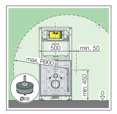
Mark the concealed socket on the left or right hand side, as required, and drill the recess hole.
