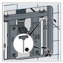
■ Insert the new gas pressure spring and attach with the Allen screws.
