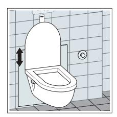
Depending on the version of the WC lid, it may be that there is contact with the wall during the height adjustment of the WC. Attaching the protective sticker prevents damage to the surface in the possible contact area on the wall and on the surface of the WC lid.
