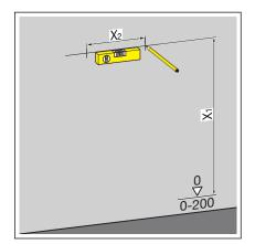
Determine and mark the fixing points.
