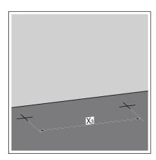
Determine and mark the fixing points on the floor.
