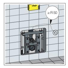
■ The radius of the hydraulic actuation must be at least 50 mm.
