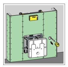
Install the concealed socket and mounting template.
