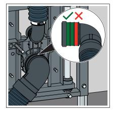
Screw the fixing elbow on the element.
