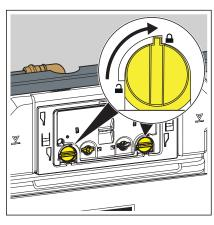
Turn the cover plate lock by 90° in a clockwise direction.
