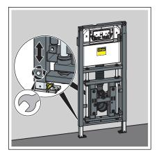
Loosen the feet of the element using a fork spanner.
