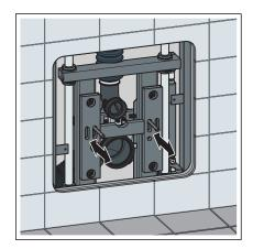
Mount the bearing surface (H support) for the cover plate flush with the wall surface.
