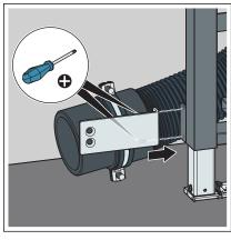
Screw the drain elbow with the fixing elbow.
