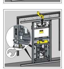
Set the height of the element by means of the feet.
