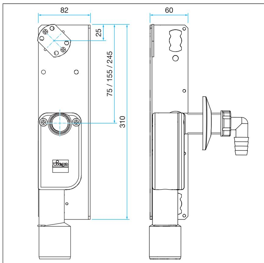
Fig. 2: Installation dimensions
