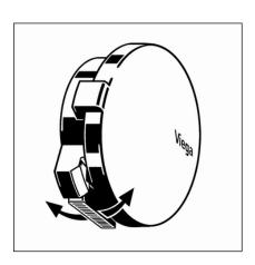
There is a regulator for the water jet on the underside of the rotatable rosette. Proceed as follows to adjust the water jet:
