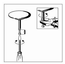
Set the valve cone with the help of the adjusting screw and counter with union nut.
