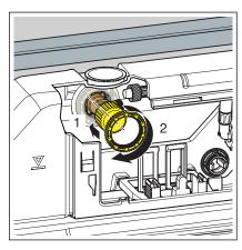
Use the lock nut to screw the corner valve and the cistern to one another.
