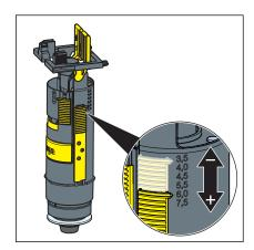
Set the large flush volume at the drain valve.
