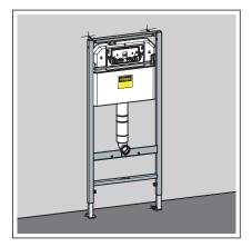
⇒ The element is attached to the wall.
