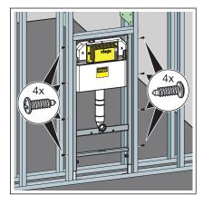
Attach the element to the support profiles using the screws supplied.
