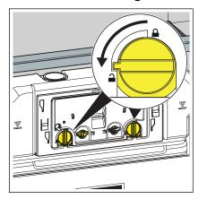
Turn the cover plate lock 90° in anti-clockwise direction.
