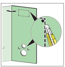
Cut out the recesses for the site protection, the revision shaft and the threaded rods.
