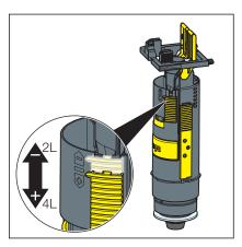
Set the small flush volume at the drain valve.
