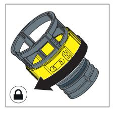
Lock the flushing throttle.
