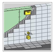
■ Clad the element with suitable gypsum cardboard cladding panels.
