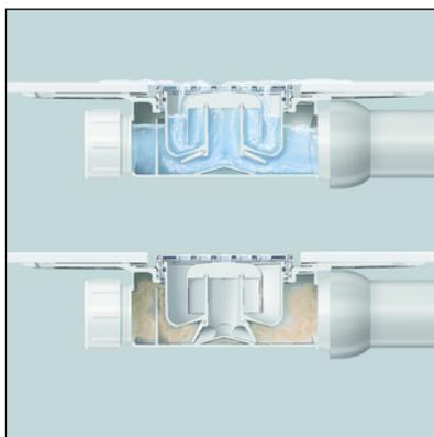
Fig. 1: Mode of operation of the odour trap
