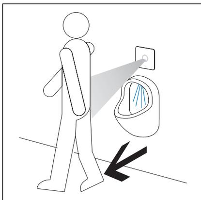
A flush cycle can also be manually actuated by placing a hand briefly in front of the sensor.
