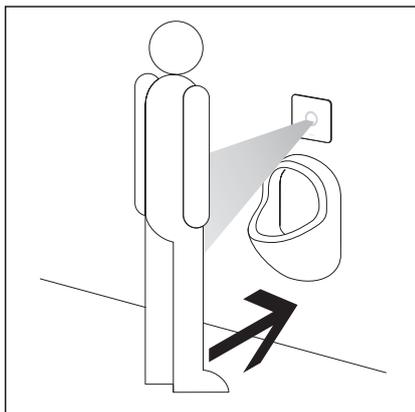
If a person leaves the detection area, a flush is automatically actuated.
