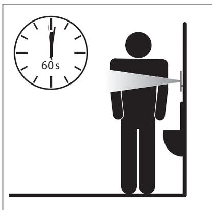
⇒ The infrared sensor is calibrated (approx. 60 seconds); the flush plate emits red light during this time.
